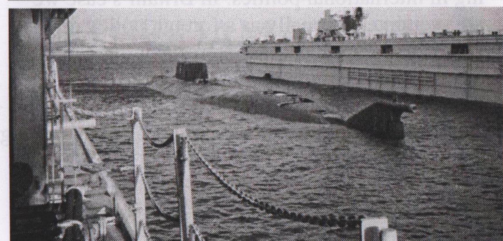
The wreck of the Kursk in dry-dock. The type of Torpedo it carried used Hydrogen Peroxide as fuel. This is so volatile it can explode if the torpedo is hit or dropped. Britain uses the same type of fuel in some of the heavy torpedoes in her navy and runs similar risks as the Russian navy
